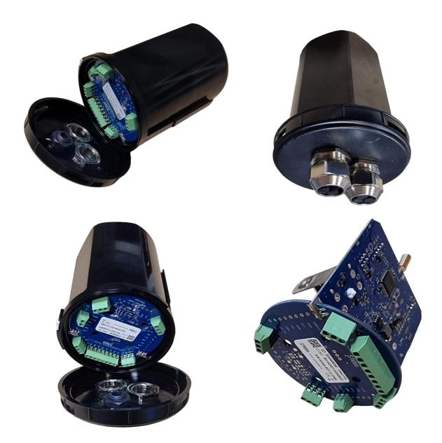
Black or gray color available. For underground installation the Goretex pressure balancer can be omitted. Plastic glands instead of metal one can be assembled. External antenna is possible upon request.
